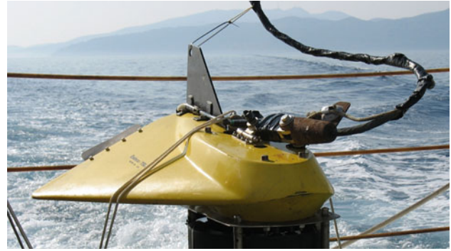
Fig. 4 Our echo repeater, used to simulate an underwater target
