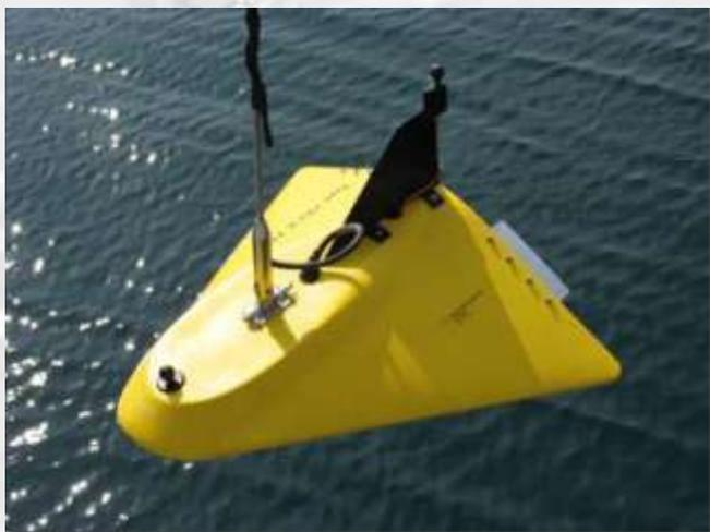
*The towed CPAM array uses a unique tetrahedral arrangement of sensors to find marine mammals.*
