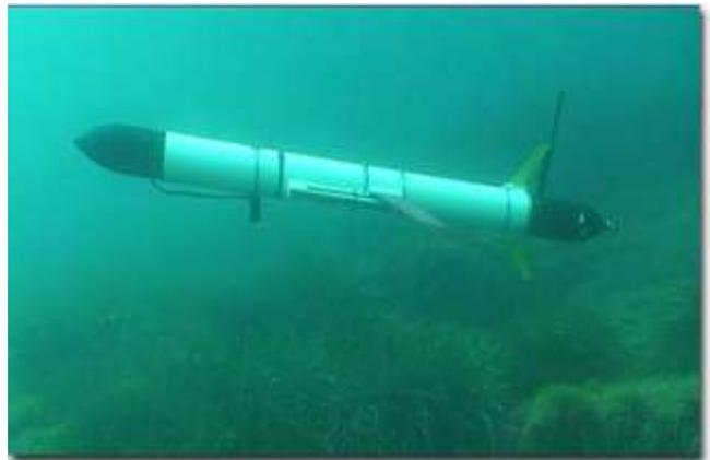
*The eFolaga hybrid AUV will be outfitted with a sensor that detects oily water.*
